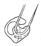
4. Cut off the tapered end as close to the mould as possible.
