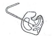
3. Pull the tubing through the mould until the tapered end has passed right through the mould. The tubing should now be at a right angle, with the tubing flat against the outside of the mould.
