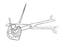
5. To adjust the tubing to the right length, place the mould in your ear and the hearing aid over the top of your ear. Ask somebody to make a mark where the tubing and end of the hook / elbow meet. Cut the tubing at this point. Another method is to hold the old piece of tubing against the new piece of tubing and cut it to the same length.
