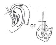
Squeeze the top of the tubing and wiggle it on over the end of the elbow / hook.
